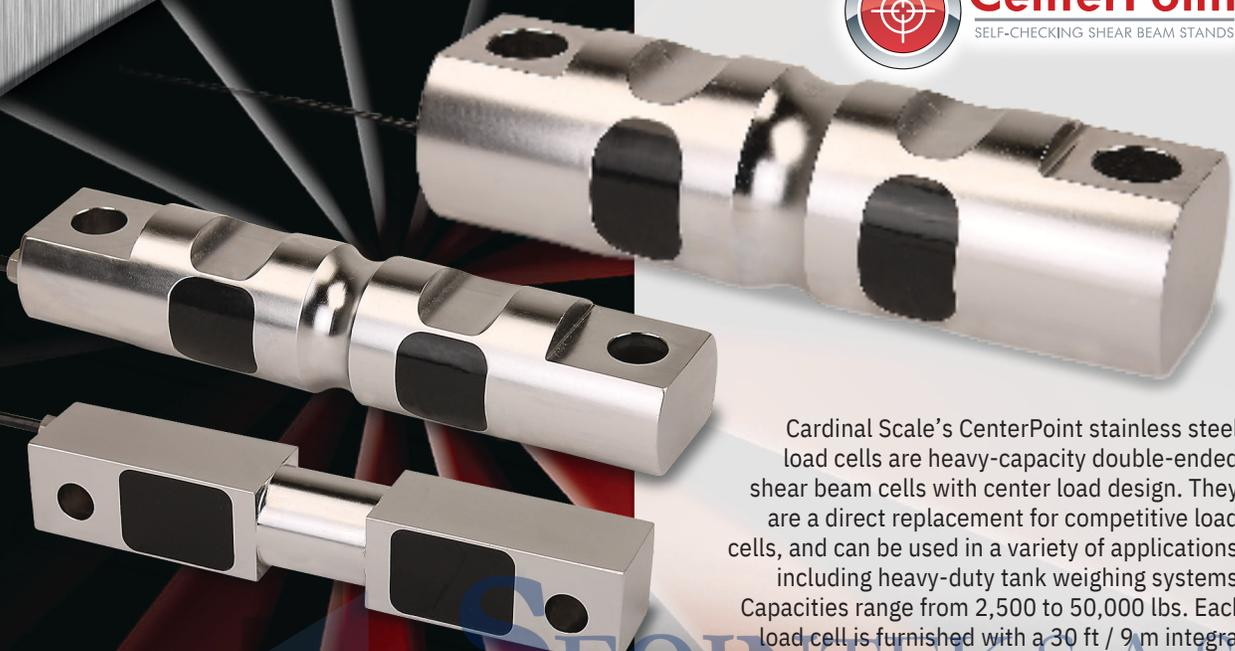
Cardinal Scale's CenterPoint stainless steel load cells are heavy-capacity double-ended shear beam cells with center load design. They are a direct replacement for competitive load cells, and can be used in a variety of applications, including heavy-duty tank weighing systems. Capacities range from 2,500 to 50,000 lbs. Each load cell is furnished with a 30 ft / 9 m integral multi-conductor cable secured by strain relief.
