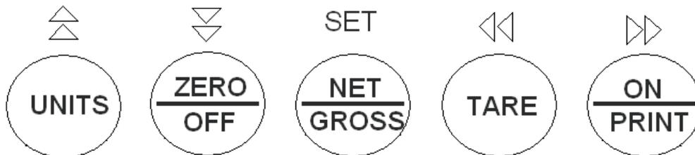
4. After setting the exact value, press the NET/GROSS key to save the ID Number value. The display will show "**SET**" momentarily, and then revert back up to A8.
